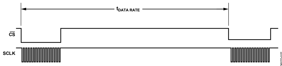
Figure 2. SPI Chip Select Timing
